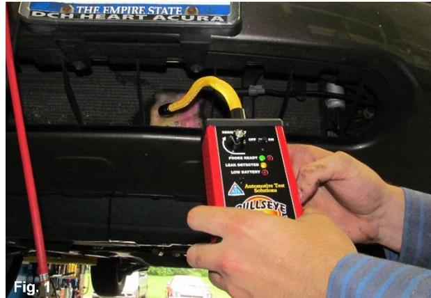
We recovered and evacuated the system and used the ATS BullsEye system, pressuring the A/C system with CO<sub>2</sub>. The CO<sub>2</sub> molecule is smaller and more easily passes through small holes, making it easier to detect. Using the special leak detector that comes with the kit, we located the area of the leak in the vehicle's condenser (Figure 1). To confirm the small leak, we sprayed the BullsEye foam on the area where the BullsEye detector had triggered.
