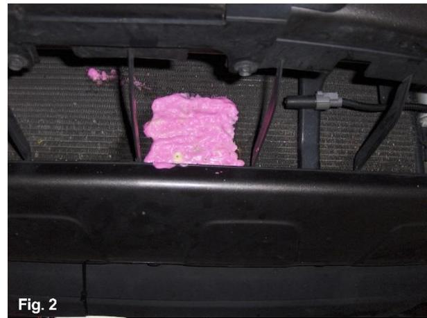
As you can see (Figure 2), the pink foam (area of no leak) reacts with the CO<sub>2</sub> and turns yellow, confirming the leak. A new condenser and receiver drier (one complete unit) later, and this customer's problem was solved!
