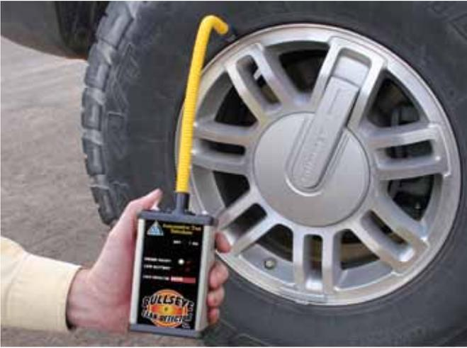
**Step 11.** Using the electronic leak detector go around the Tire and wheel to identify the leak site area. While moving the CO2 probe tip around the system it is best to keep the CO2 sensor face perpendicular to the surface being tested.
