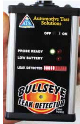
**Step 12.** When CO2 gas is detected the LED display bar is activated along with the audio alert (loud beeping noise). Once the detector has sensed CO2 the alerts will continue for about 10 to 40 seconds; **Note:** *Remove sensor from leak site area and let the unit stop beeping on its own.* Once the detector has stopped beeping you can now retest the leak site area with the CO2 detector.
