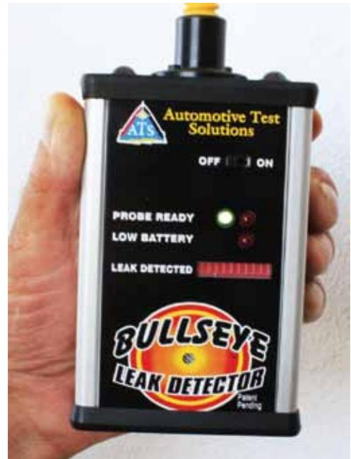
**Step 2.** Remove electronic leak detector from kit and turn on unit, allow unit to warm up the CO2 sensor tip. When unit is ready the red light will shut off and the green ready light will turn on, this will take about 90 seconds. For best results the leak detector CO2 sensor should be allowed to fully warm up for about 5 minutes.
