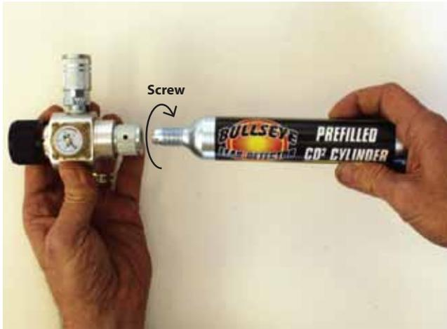
**Step 6.** Remove high pressure regulator with adaptor from kit and screw CO<sub>2</sub> cylinder to high pressure regulator. **Note:** *Due to the volume in tires it will be better to use a larger 24oz paint ball container this is available at all department or sporting good stores stocking paint ball supplies.*
