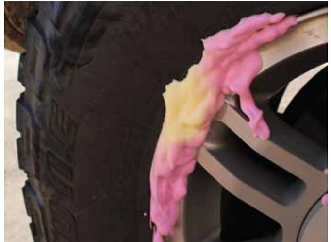
**Step 14.** The Bullseye Leak Seeker Solution foam will turn from red to yellow in color at the leak site and may also bubble. This will make it very easy to identify the exact location of the leak site.
