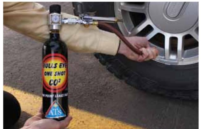
**Step 9.** Fill the tire using an air chuck (not included) with CO<sub>2</sub> and pressurize the tire to the correct pressure shown on the tire side wall.
