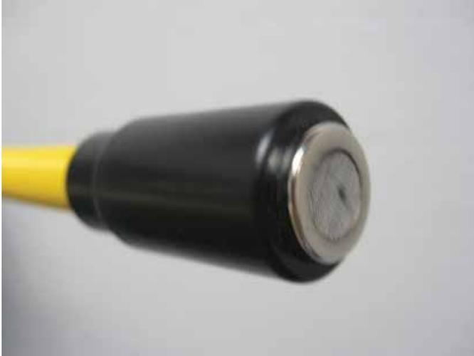
**Note:** Never directly hit or drop the leak detector on the CO2 sensor tip, this will cause the sensor to become damaged! Do not get Leak Seeker Solution directly on the CO2 sensor tip!
