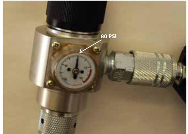
**Step 7.** Adjust the high pressure regulator by turning the knob on top clockwise until the gauge on the front of the regulator reads 80 PSI.
