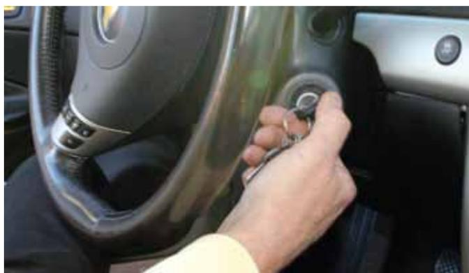
**Step 9.** Turn on the vehicles ignition key to the on position. **Do not start the engine.** It is a good idea to connect a battery maintainer or battery charger to insure the battery voltage is stable for the entire testing time.
