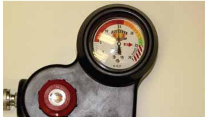
**Step 12.** If the fuel containment system has more pressure than 15" of H<sub>2</sub>O, the vent valve may not open. This means if you are testing the valve to see if it can open and close and still seal; the test must be done with less than 15" H<sub>2</sub>O in the system.
