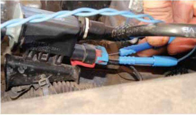
**Step 16.** Now back probe the purge solenoid. The purge solenoid will have two wires power and control; either back probe can be connected to either purge solenoid wire. The purge solenoid is normally closed. Open and close the purge control valve and watch to see if the pressure is stable or leaking after the valve is actuated
