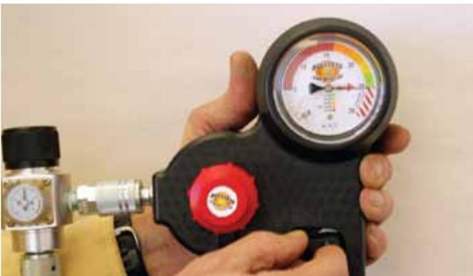
**Step 13.** Actuate the vent valve in order to close it, now open the low pressure regulator shut off valve so the CO<sub>2</sub> will pressurize the fuel containment system.
