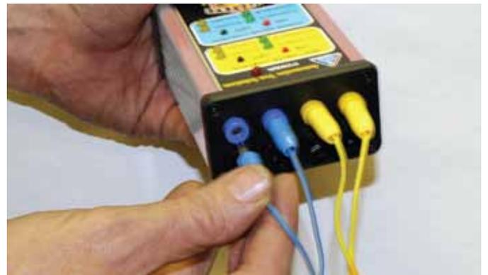
**Step 14.** Take out the blue lead and connect lead to blue banana plugs on top of the smart control unit.
