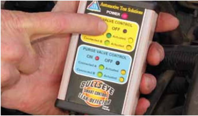
**Step 11.** To actuate the solenoid push the red on button, and to un-actuate the solenoid push the black off button.
