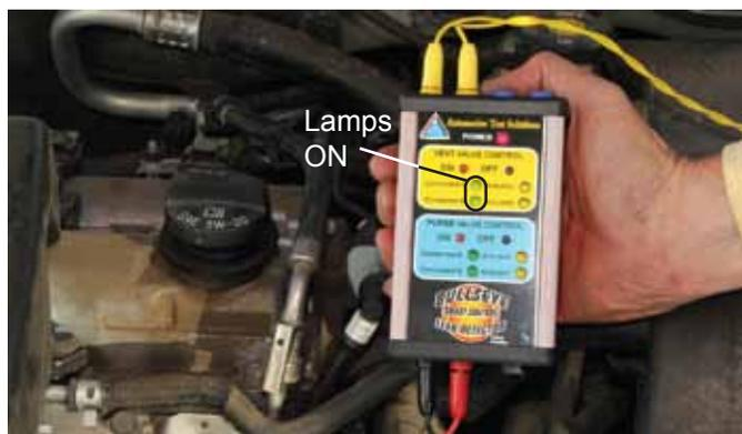
**Step 10.** If the back probes are connected to the solenoid wires the green connected A lamp, and connected B lamp will be on. If one or both lamps are not on, check the connections at the solenoid; make sure there is power supplied from the vehicle to the solenoid; additionally if the fuse(s) in the smart control is blown the lamp will not be on (these are located on top of the smart control box next to the yellow banana plugs).
