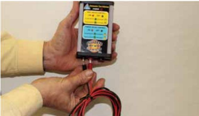
**Step 3.** Install red and black power lead to smart control bottom banana jacks; red to red, black to black.
