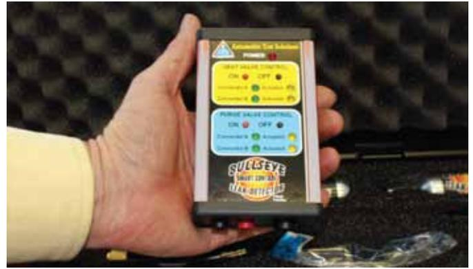
**Step 2.** Remove smart control from case. This Smart Control unit will only work to control electrical solenoids.
