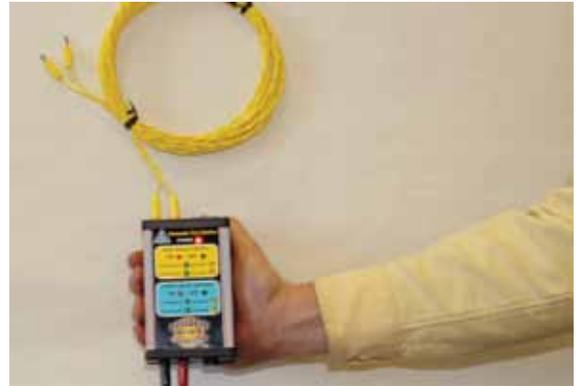
**Step 6.** Take out the yellow lead and connect lead to yellow banana plugs on top of the smart control unit.
