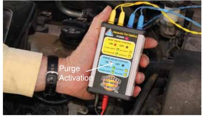
**Step 17.** Once all testing is finished actuate the purge control so the pressure in the fuel containment system is dumped in to the intake manifold of the engine. **Note:** this may cause a hard start condition.
