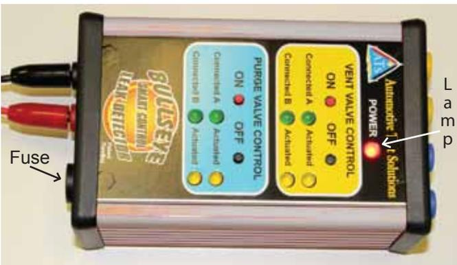
**Step 5.** Make sure that the red power lamp is on indicating the smart control has power and is ready to use. **NOTE:** if the fuse located on the bottom of the smart control is blown the power lamp will not be on.
