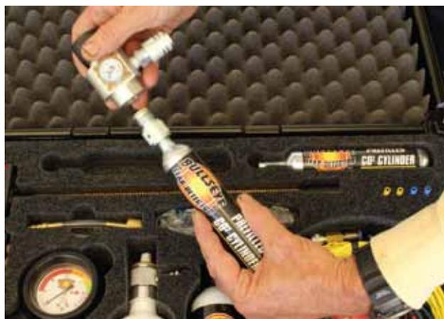
**Step 30.** Unscrew the high pressure regulator from the 90 gram CO2 cartridge and adaptor.
