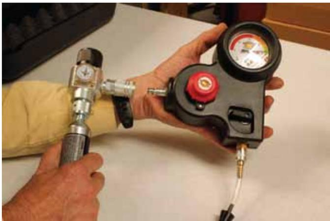
**Step 27.** Disconnect the high pressure regulator from the low pressure regulator.
