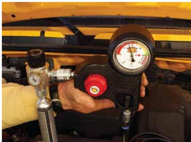
**Step 16.** Watch the low pressure gauge for about 20 seconds and make sure that the pressure does not start to increase. If the pressure starts to rise up this indicates that there is a restriction in the system that you will need to repair before going to the next step. **After the 30 second time make sure to close the CO<sub>2</sub> shut off valve.** If there was no restriction in the system go to the next step.
