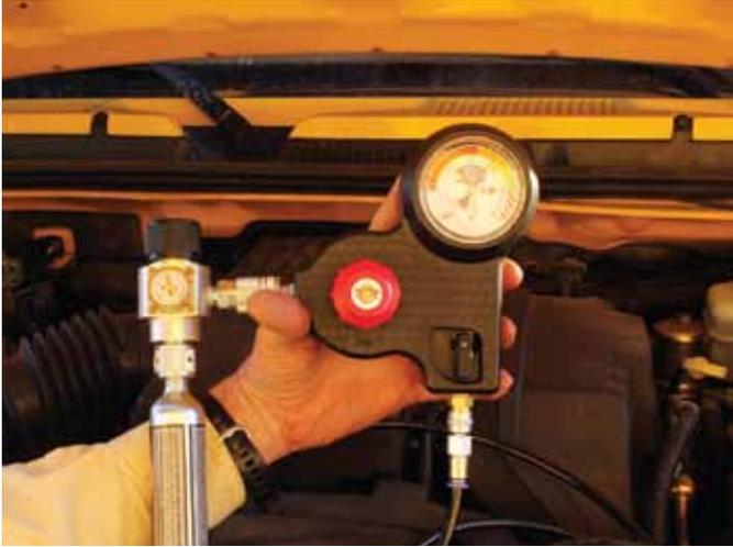
**Step 19.** If there is not a large or gross leak present, allow the system to fill with pressure for about 4-6 minutes.
