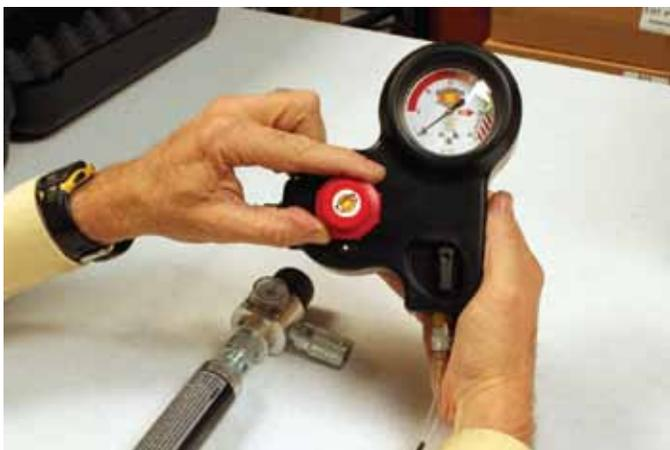
**Step 29.** Once the pressure has been drained turn the low pressure adjustment knob counterclockwise until it hits it's stop. Now unit is ready for storage.
