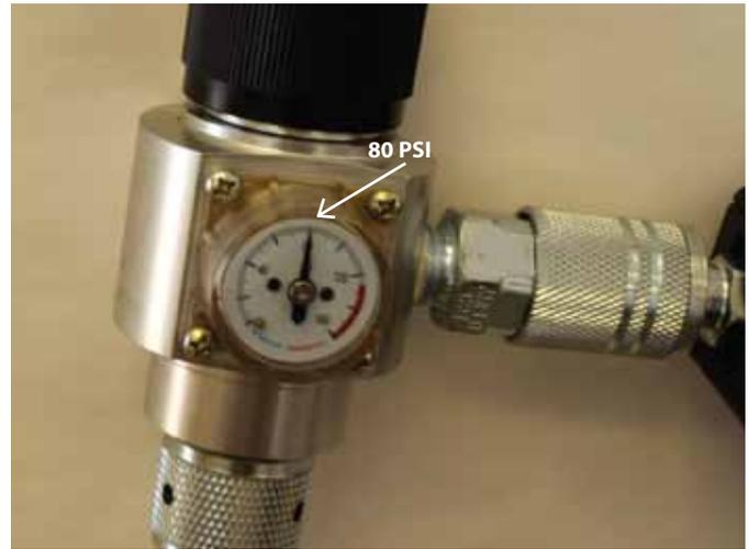
**Step 11.** Adjust high pressure regulator to 80 PSI by turning adjustment knob and watching high pressure gauge.
