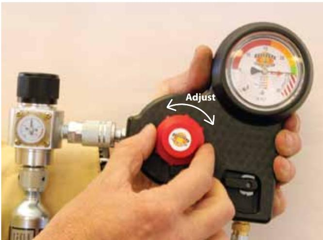
**Step 12.** Check and adjust low pressure regulator, red knob on low pressure gauge assembly, to 25" H<sub>2</sub>O.
