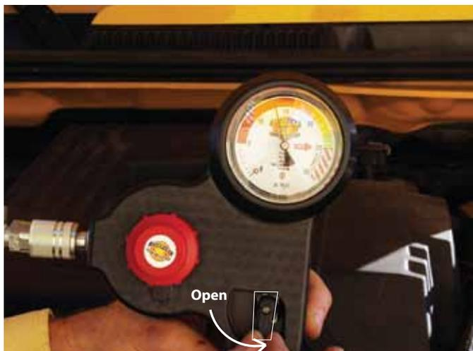
**Step 15.** Now that the Bullseye CO<sub>2</sub> system is connected to the vehicle open the shut off valve that is located on the low pressure gauge assembly, this will allow CO<sub>2</sub> to flow into the vehicle.
