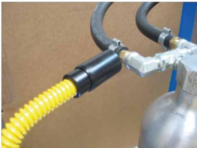
**Step 23.** Using the electronic leak detector go around the system to identify the leak site area. While moving the CO2 probe tip around the system it is best to keep the CO2 sensor face perpendicular to the surface being tested. **Note: If tip is bumped against the surface being tested the detector may momentarily go off, this false alert will go off right away. If the leak detector senses CO2 gas the alert will stay on for 10 to 40 seconds.**
