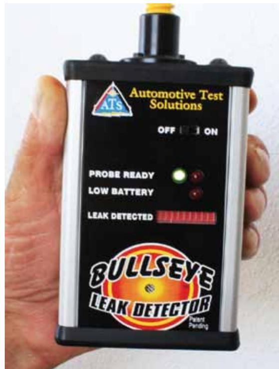
**Step 2.** Remove electronic leak detector from kit and turn on unit, allow unit to warm up the CO2 sensor tip. When unit is ready the red light will shut off and the green ready light will turn on, this will take about 90 seconds. For best results the leak detector CO2 sensor should be allowed to fully warm up for about 5 minutes.
