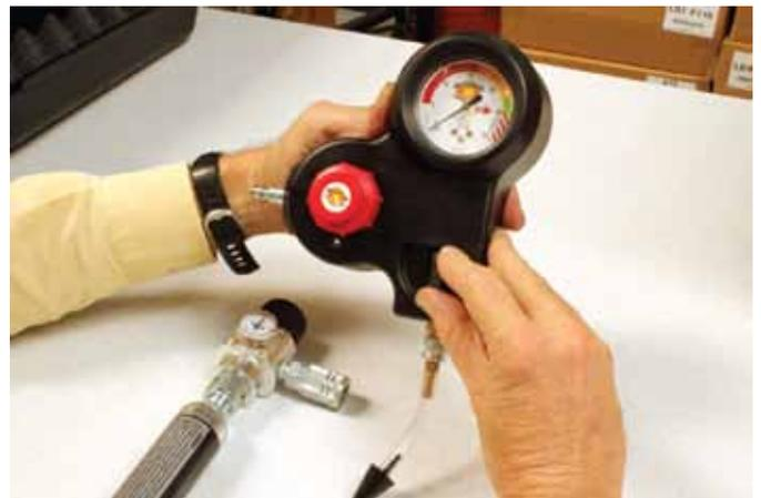
**Step 28.** With the EVAP Hose connection installed on the low pressure regulator open the check valve and drain all remaining pressure from low pressure regulator.
