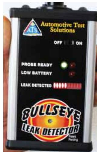
**Step 24.** When CO2 gas is detected the LED display bar is activated along with the audio alert (loud beeping noise). Once the detector has sensed CO2 the alerts will continue for about 10 to 40 seconds; **Note: Remove sensor from leak site area and let the unit stop beeping on its own.** Once the detector has stopped beeping you can now retest the leak site area with the CO2 detector.
