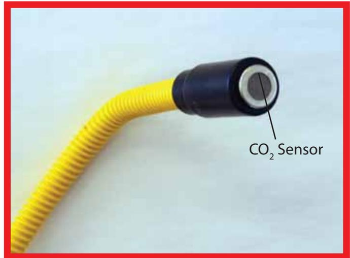
**WARNING!** Do not allow leak seeker foam to get on CO<sub>2</sub> sensor at end of yellow flex tube! This will damage CO<sub>2</sub> sensor and will require the CO<sub>2</sub> sensor to be replaced.
