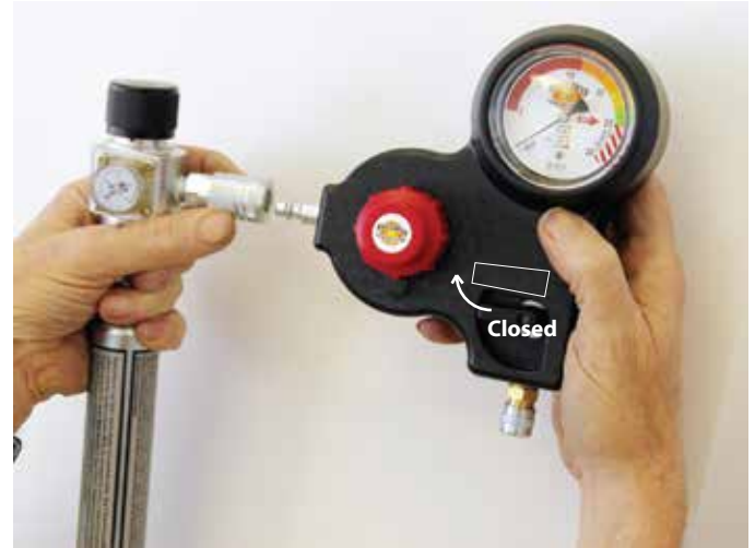
Step 7. Remove low pressure gauge assembly from kit and attach it to the high pressure regulator, make sure the shut off valve is closed.
