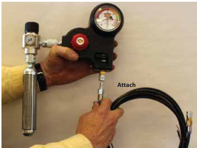
Step 8. Remove black CO2 fill hose from kit and attach it to the low pressure gauge assembly.
